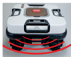
RADAR rilevamento ostacoli RADAR for obstacle detection
